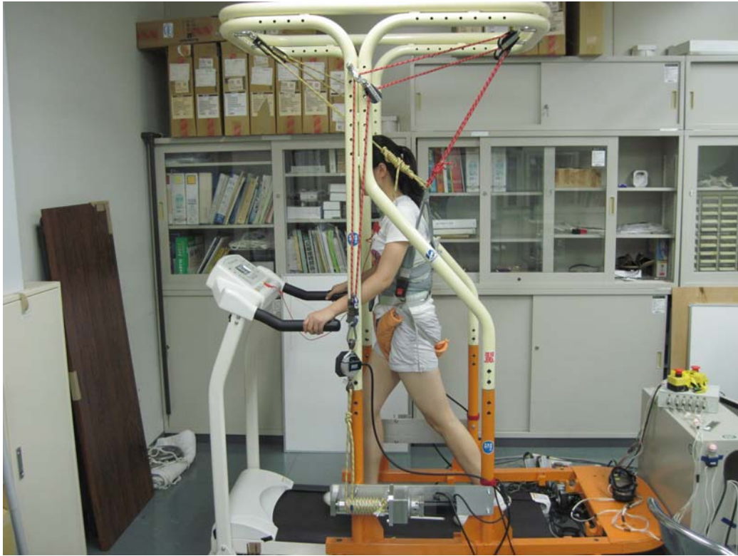
Fig.5-1. Prototype of a volunteer in the gait rehabilitation experiment.
