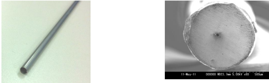
Figure 3.4 A stainless steel tube and the surface of orifice gas nozzle
