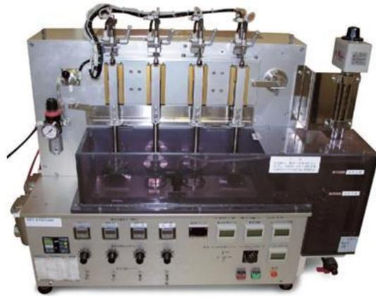
Figure 3-2. Impact abrasion testing machine.
