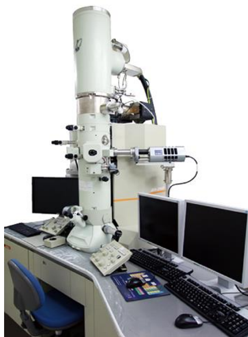
Fig. 2.8 The JEOL-2100F TEM system.
