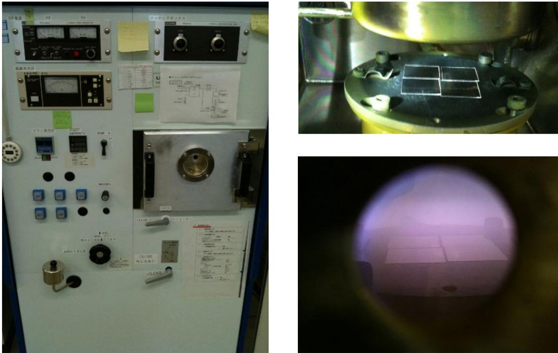
Fig. 3-5 Sputtering machine RFS-200
