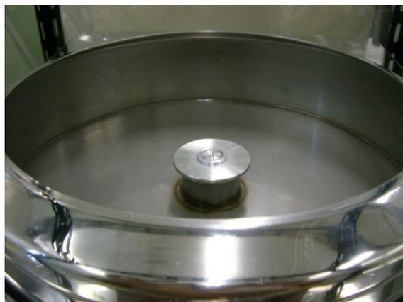
Fig. 2-4 Spin-coating machine
