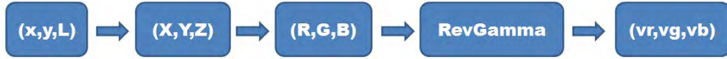
Figure 4.4: The flowchart of the kernel procedure xyL2Vrgb . The expectative luminance and chromatic coordinate (x,y,L) is transformed into the control values of three guns of the CRT (vr,vg,vb) .
