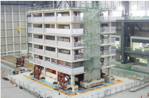
Fig. 1.13 A full-scale six-story RC wall-frame building tested at E-Defense [17]
