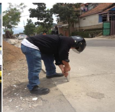
Rebound Hammer test
