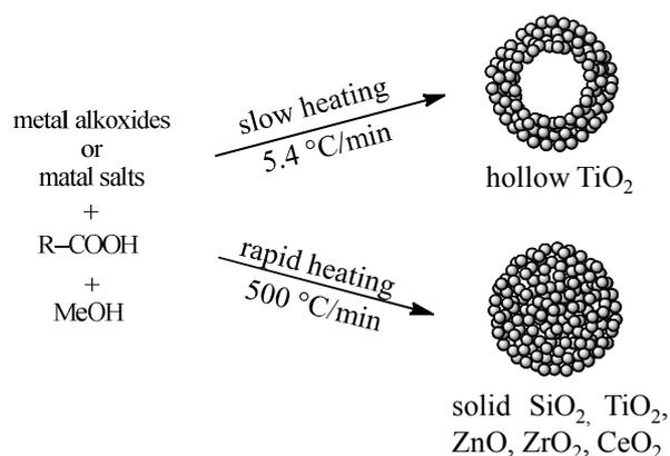
**Figure 1.** Synthesis of solid and hollow MARIMO assemblies by one-pot single-step method.
