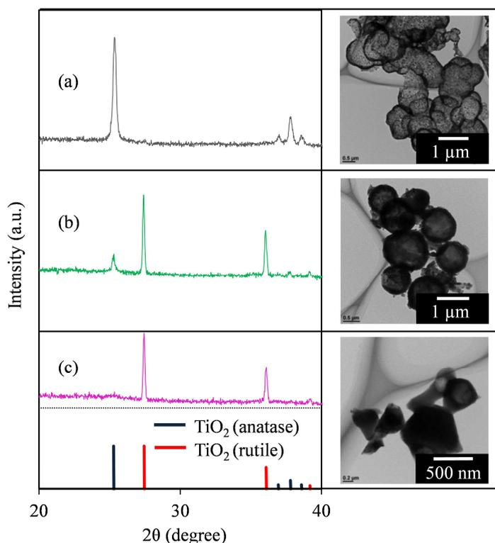
**Figure 3.** XRD patterns (left) and TEM images (right) of (a) Al/Ti-0.50, (b) Al/Ti-0.25, and (c) Al/Ti-0.05 hollow composite assemblies after calcination at 1,000 °C for 1 h.
