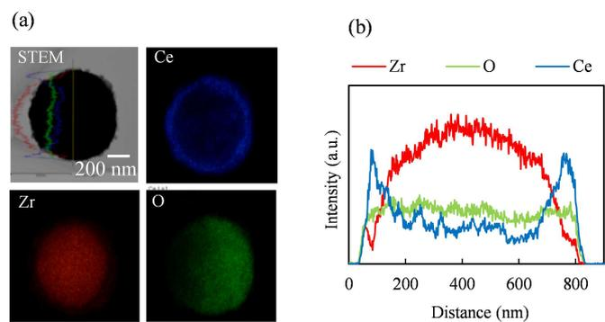
**Figure 7.** EDX (a) mapping images and (b) line scans of ZrO<sub>2</sub>@CeO<sub>2</sub> core-shell MARIMO composite assemblies.
