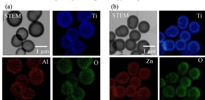
**Figure 2.** STEM and EDX mapping images of (a) Al/Ti-0.20 and (b) Zn/Ti-0.20 hollow MARIMO composite assemblies.
