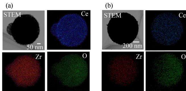
**Figure 5.** STEM and EDX mapping images of (a) Ce/ZrO<sub>2</sub>-0.50 and (b) CeO<sub>2</sub>-ZrO<sub>2</sub>-SH MARIMO composite assemblies.
