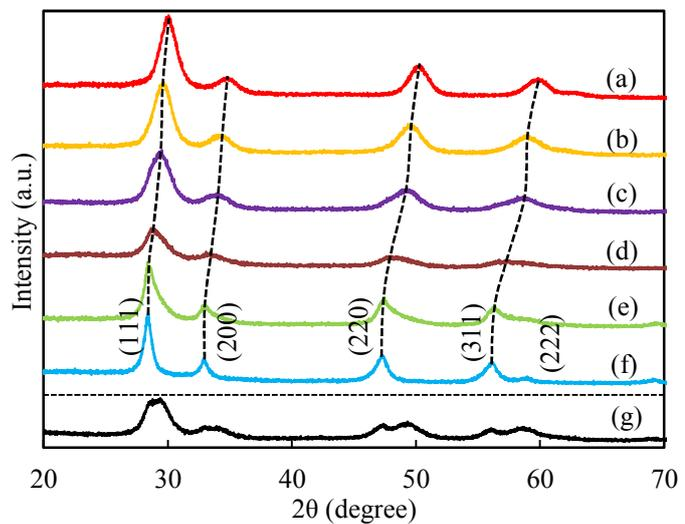
**Figure 6.** XRD patterns of MARIMO NPs: (a) ZrO<sub>2</sub>, (b) Ce/ZrO<sub>2</sub>-0.25, (c) Ce/ZrO<sub>2</sub>-0.33, (d) Ce/ZrO<sub>2</sub>-0.50, (e) Ce/ZrO<sub>2</sub>-0.66, (f) CeO<sub>2</sub>, and (g) CeO<sub>2</sub>-ZrO<sub>2</sub>-SH
