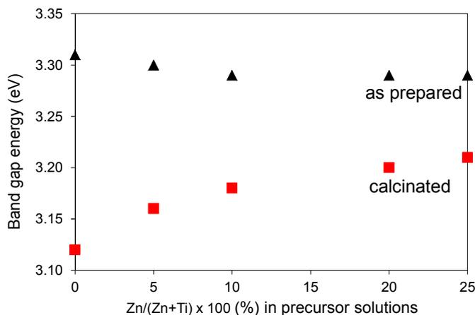
**Figure 4.** Plots of band gap energies of  $\text{ZnO-TiO}_2$  hollow composite assemblies versus the initial molar fractions of Zn in precursor solutions.
