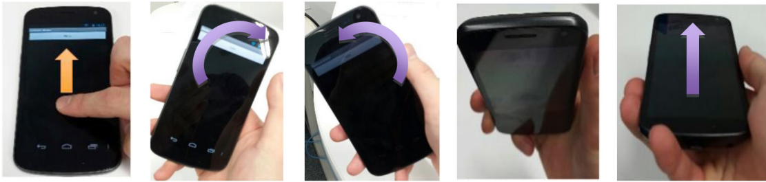
Figure 3.5: Motion gesture interfaces of making a call. (1) A flick gesture to browse phone book, (2) Flip motion to right is used to browse contact, (3) Flip motion to left is used to browse previous contact, (4) Flip backward to select the contact and make call, (5) Flip forward to hang-up the call.
