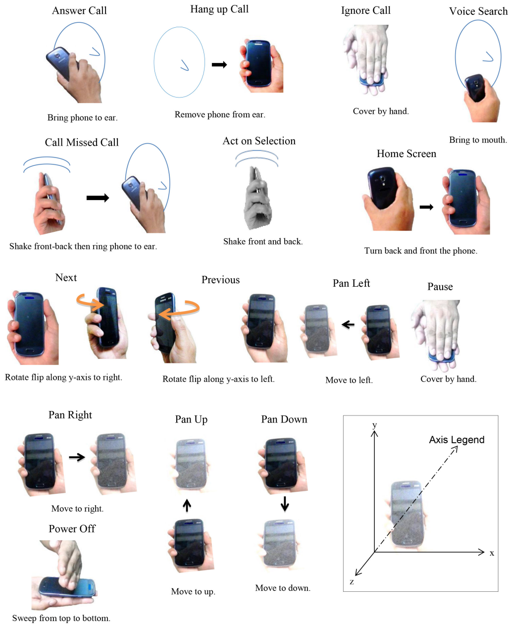
Figure 3.2: A User-defined gesture set. Commands for zoom in and zoom out are not included due to the lack of agreement among the participants. Blue curve shows front-back movement of shake, black arrow indicates state change of the phone or direction of movement, and brown-bold arrow indicates the direction of rotations.
