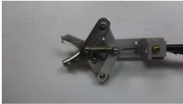
Figure 1-4 Cutter – pincer end-effector, which was chosen for this study
