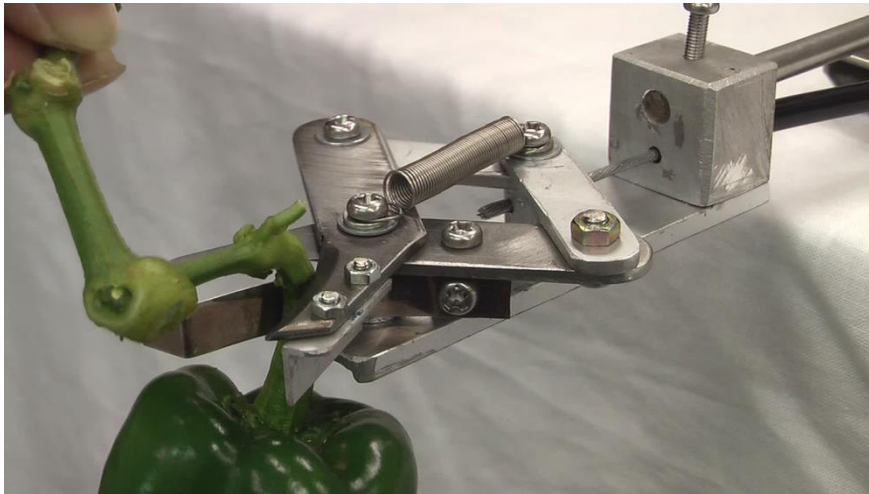
Figure 4-7 The end-effector used by the harvesting robot.
