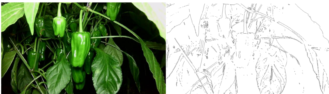
Figure 2-6 Example of texture extraction method using edge detection (Prewitt method).
