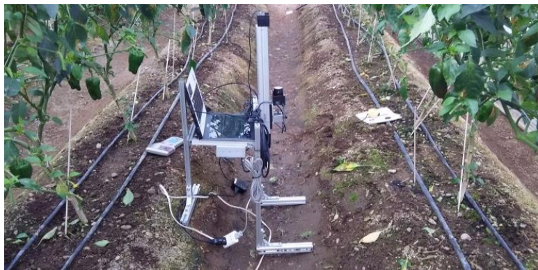
Figure 3-2 Pose estimation setup for the greenhouse test
