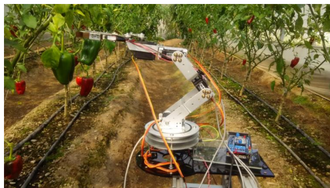
Figure 4-26 Setup for the movement and greenhouse tests
