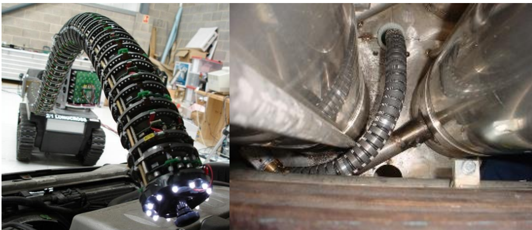
Figure 5-9 Robot with a continuum manipulator on the left, and during nuclear site examination test on the right [OC Robotics].
