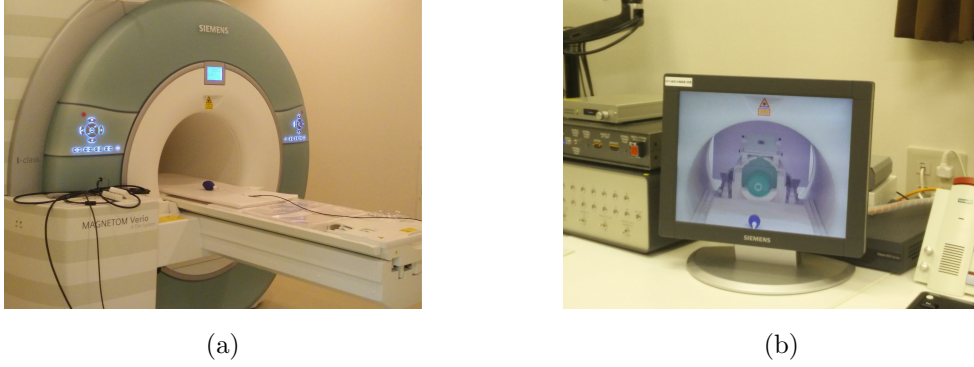
Figure 4.10: Experiment in the fMRI room and result images. a) The pneumatic device was put on the fMRI bed to be tested, b) a view of the pneumatic device while the fMRI was running.
