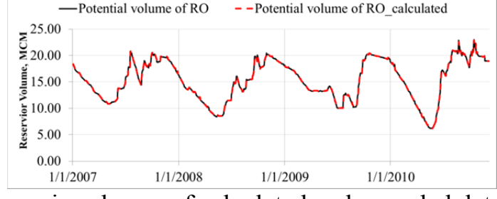
(e) Reservoir volumes of calculated and recorded data at RO
