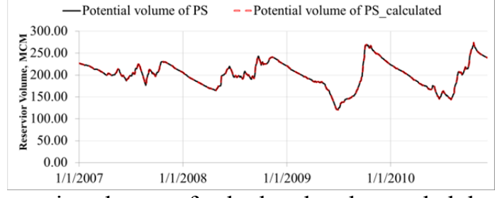
(d) Reservoir volumes of calculated and recorded data at PS
