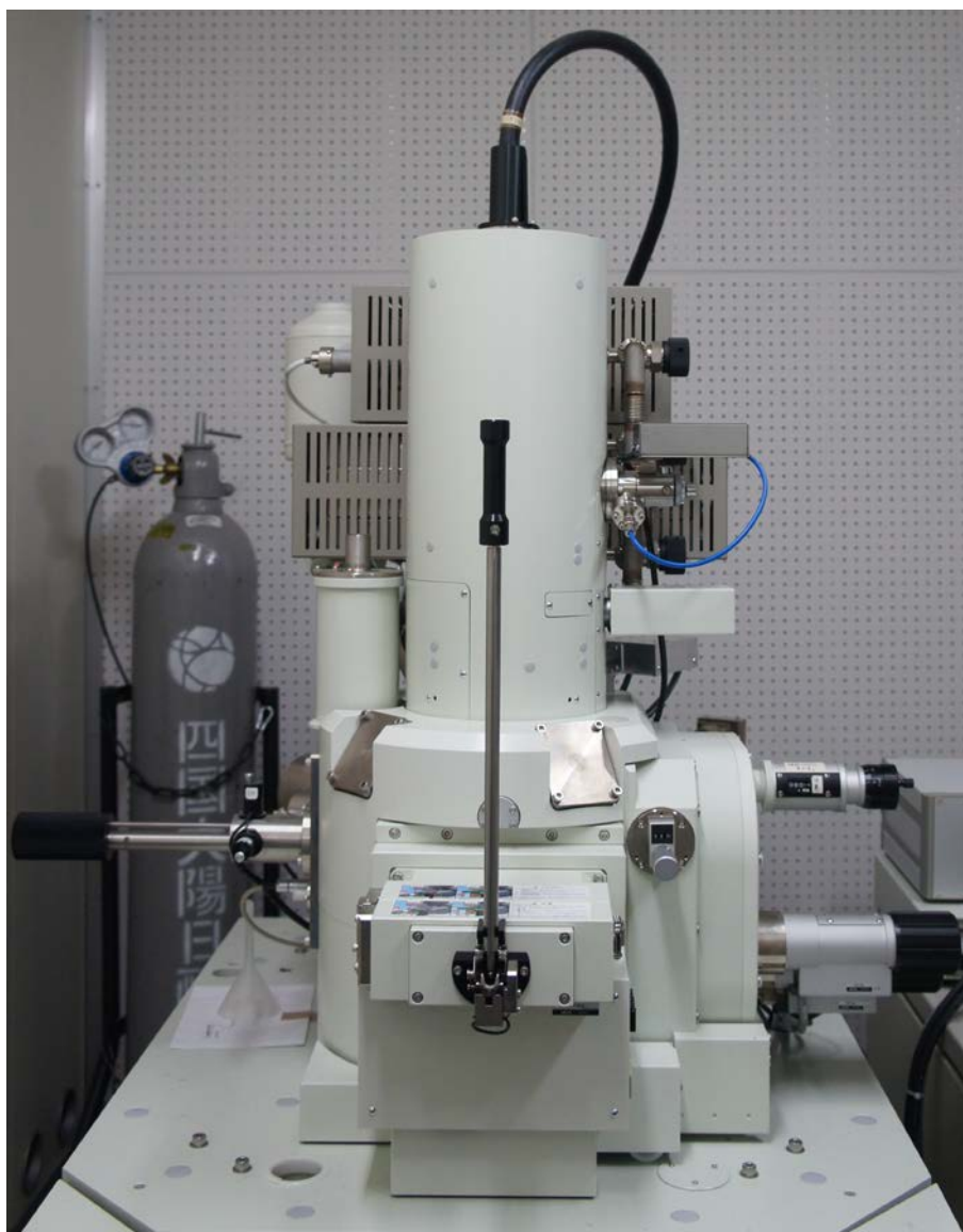
Figure 3.3. Field Emission Scanning Electron Microscope JEOL JSM-5310.
