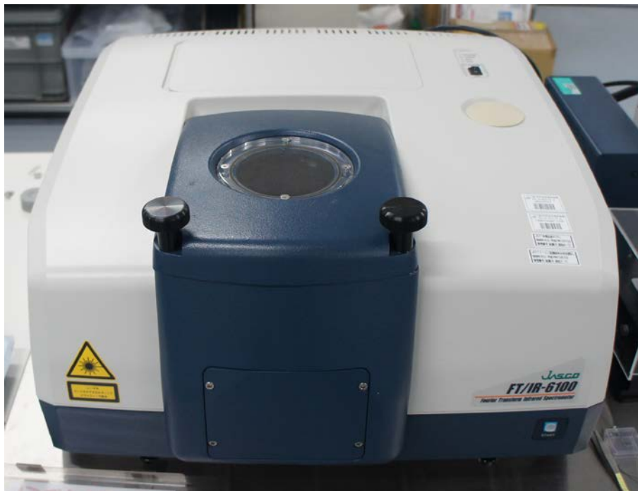
Figure 3.8. Fourier transform infrared spectrometer (FT-IR) JASCO FT/IR-6100.
