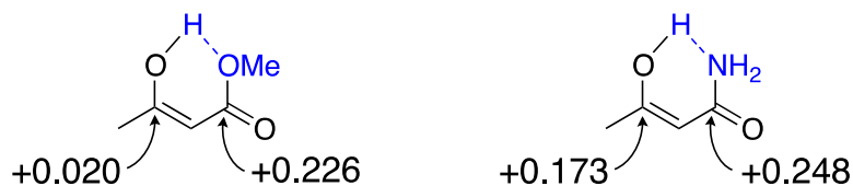
Figure 2. Estimated electrophilicities of carbonyl groups using DFT calculation using 6-31G + .
