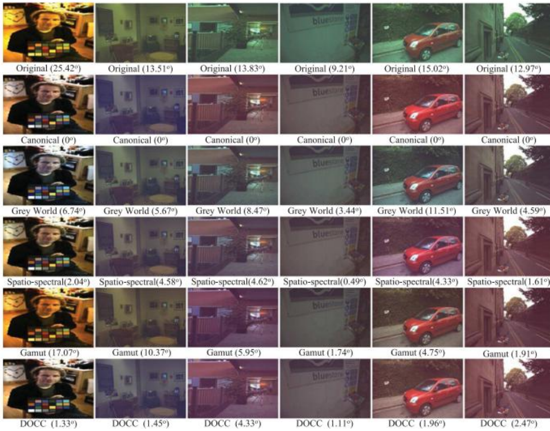
Figure 1. 40 Some examples of indoor and outdoor images from Gehler-Shi dataset corrected with multiple methods. From Gao (2015).
