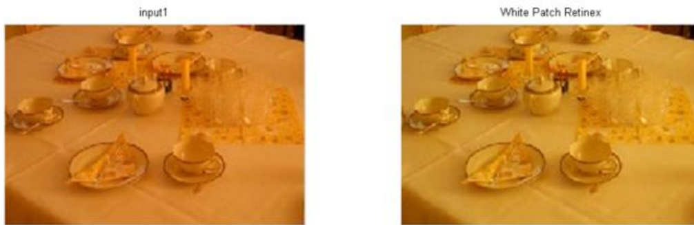
Figure 1. 34 The white patch retinex algorithm is used to perform the color adjustments for the input image, the result is show in the right side. From Ebner(2007).
