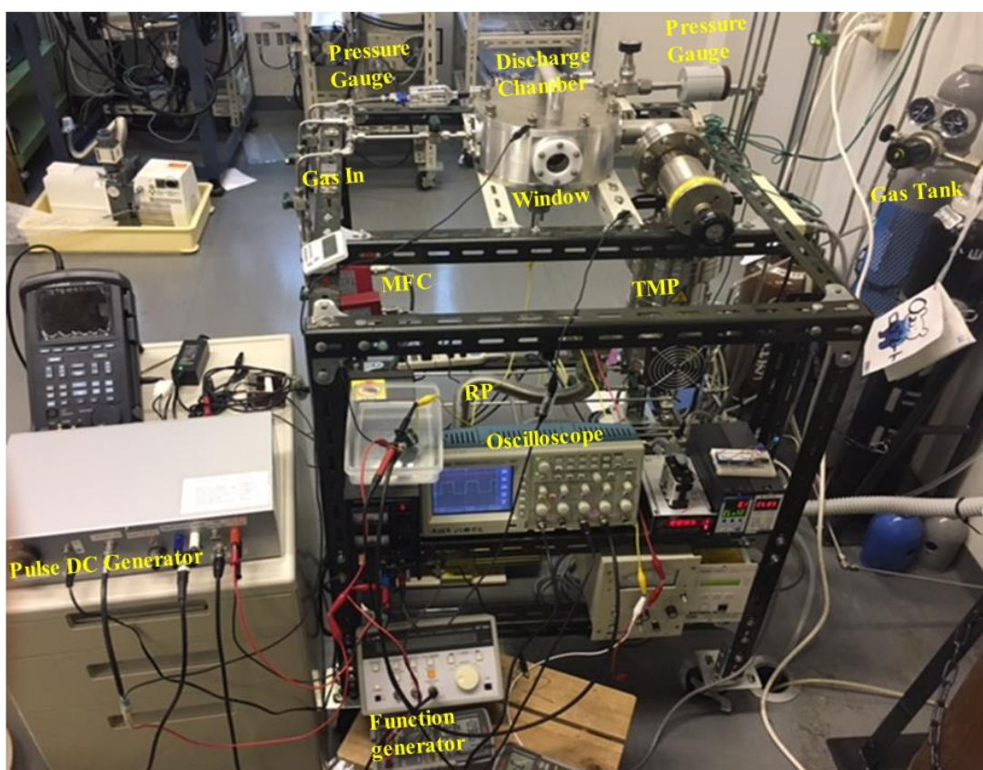
Figure 3.1. Picture of the developed pulsed DC plasma CVD system
