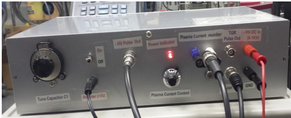
Figure 4.10. Image of the fabricated Pulsed DC Generator (PDG)
