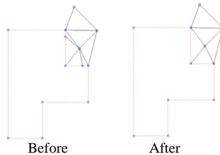
Fig7 Delete the minute distance point of building
