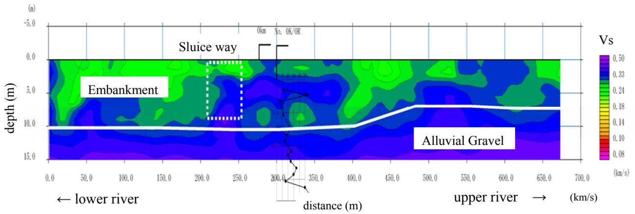
Fig. 7 S-wave velocity contour
