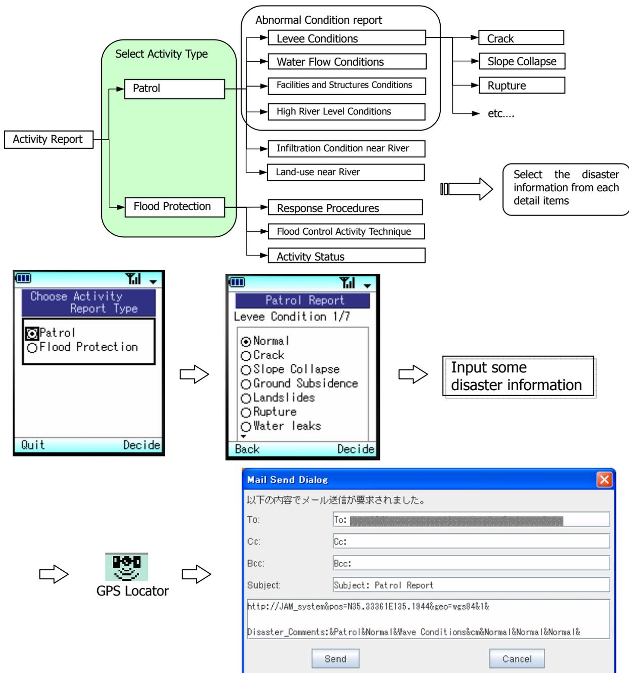
Figure 3 Input Support Application written by Java Programming
