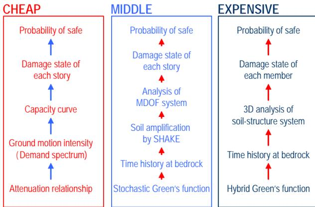
Figure2. Example of current simulation models for the computation of the probability of safe
