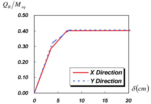
Figure5. Capacity curve for the industrial building
