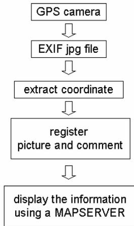
**Figure 1.** The proposed data acquisition method for field surveying
