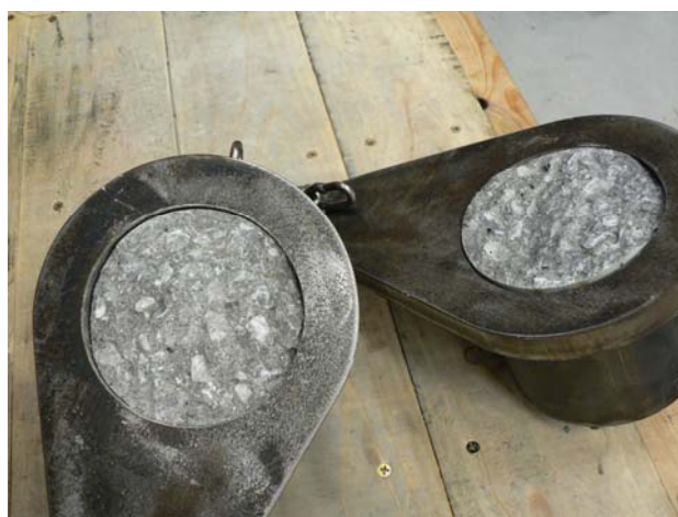
Fig. 14 Shear failure of jointless specimen of concrete by the apparatus
