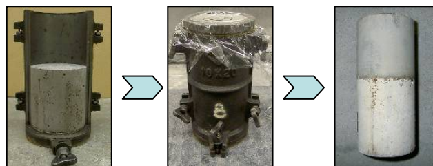
Fig. 9 Specimen for bond strength: common in both tensile and shear bond strength; upper: self-compacting mortar; lower: base material concrete (conventional concrete)
