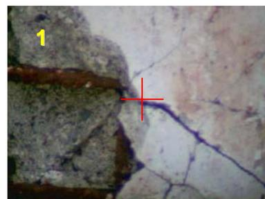
Figure 12 Crack target 1 measured by the image
