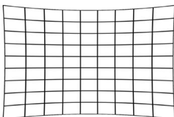
Figure 1. Radial lens distortion
