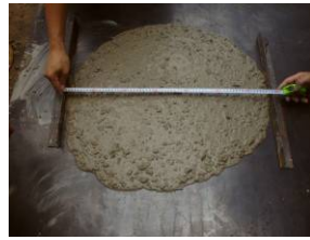
Slump flow test
