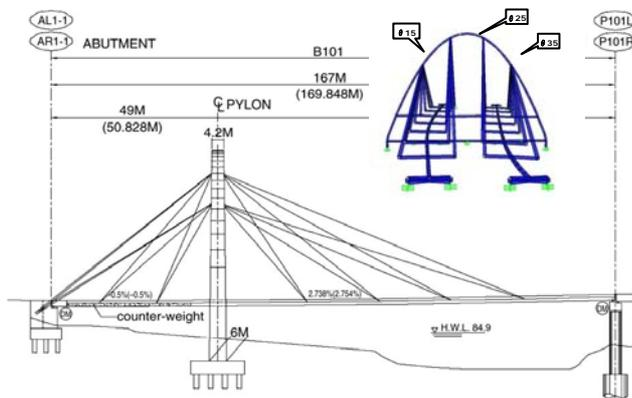
Fig. 1. Elevation of the Mau-Lo-Hsi Cable-Stayed Bridge.
