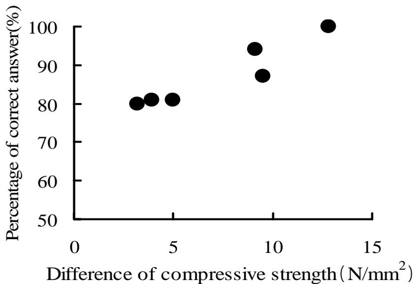
Fig.15 Relation between percentage of answer distinguishing correctly and difference of actual compressive strength of concrete (Specified mix is shown in Table 4)
