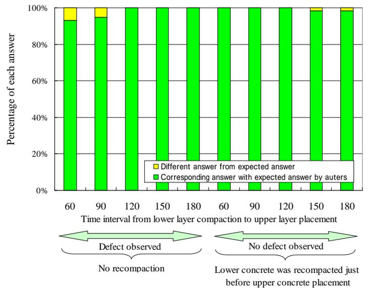
**Fig.13 Result of visual test for Sand Streak**
