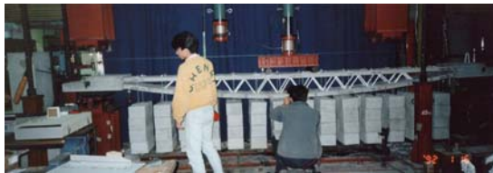
Fig.14 Suspension cable supporting roads, externally anchored during construction, and afterwards self-anchored, (Yokohama National University)
