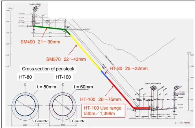
**Fig.4.15 Application of HT-100 for Penstock**
