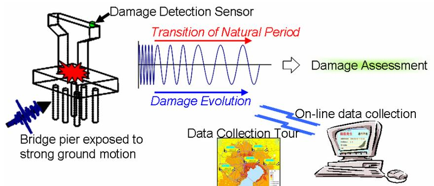
Fig.8 Damage Evaluation based on Natural Period Change
