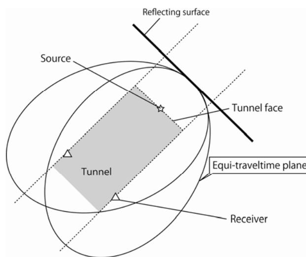
**Figure 2.5 Imaging of a reflecting plane by tangential planes of two ellipsoids.**
