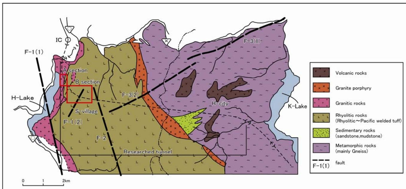
Figure 2.1 Locality and Geological map of researched tunnel.
