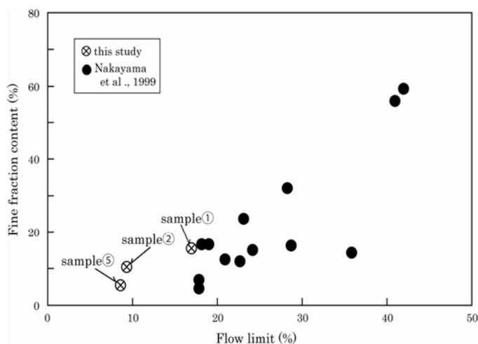
**Figure 2.4 Relation between the fine fraction content and the flow limit**
