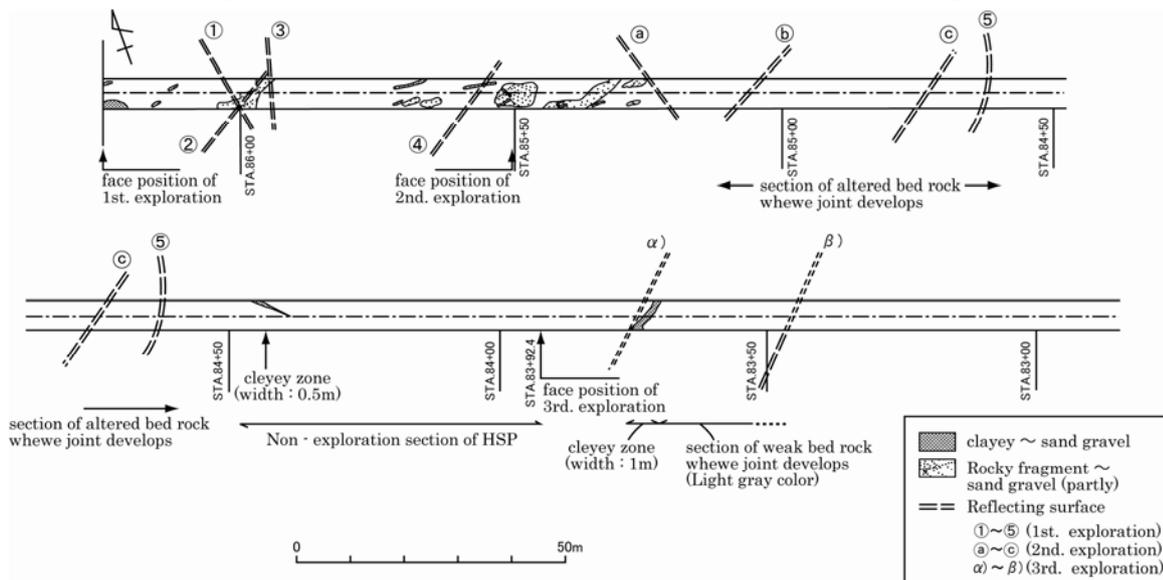
**Figure 2.7 HSP exploration result and actual excavation result**
