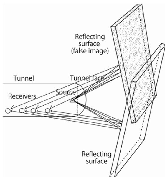
**Figure 2.4 Conceptual diagram of seismic imaging ahead of tunnel face.**
