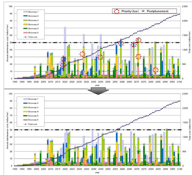
**Fig.7** Case of application of facility priority assessment to LCC leveling
